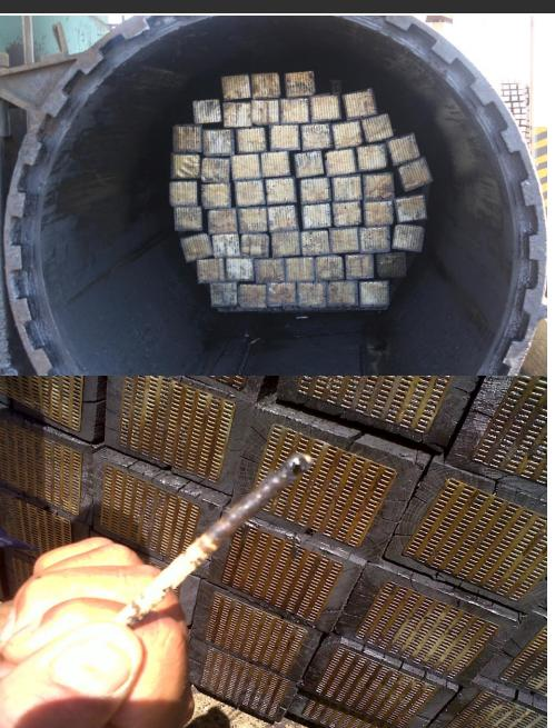
All our ties are dual treated with borate + creosote, incised, and end plated according to AREMA & AWPA standards.
